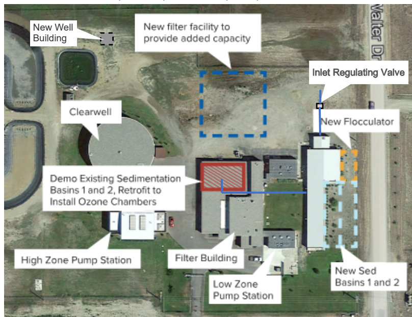
Figure 10: Proposed Facility Modifications for Capacity Expansion
