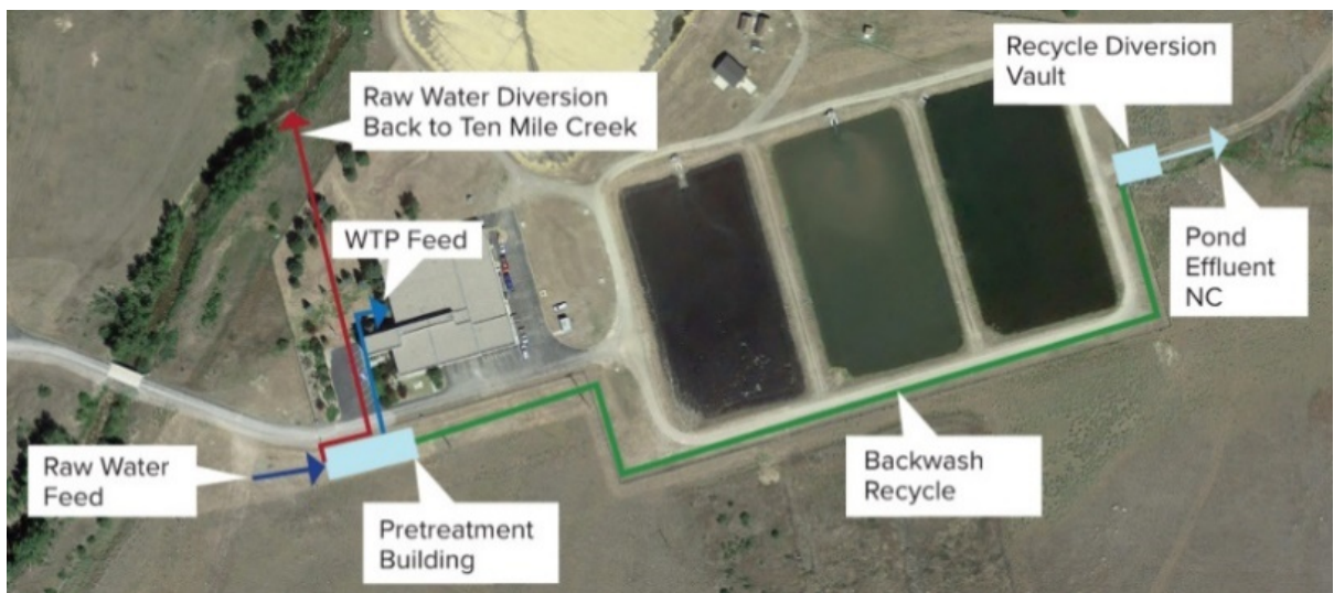
Figure 4: Proposed TMWTP Process Layout with Backwash Recycle
