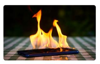
When improperly handled, overcharged, or the battery becomes defective or damaged, lithium-ion batteries have the potential to swell, overheat, combust, and cause high-heat scenarios known as "thermal runaways," which cause thousands of fire incidents each year.
