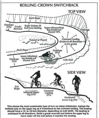
Switchback: Switchbacks are necessary for making turns on steeper terrain and are much "tighter" than climbing turn. The South Hills trail system has many examples of switchbacks both good and bad. See the IMBA manual for a good description of switchback construction.
