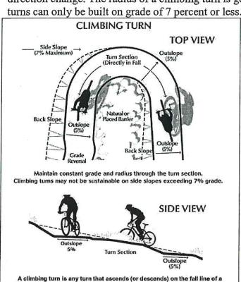
sideslope. Improve sustainability by placing climbing turns on gentle slopes and using grade reversals to drain water above them. Climbing turns should have a large turning radius and barriers between legs to prevent shortcutting.
