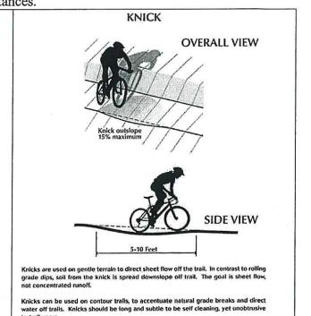
Knick: Knicks are gentle fanned shaped depressions about five to ten feet in diameter built into the trail that open towards the downhill side of the trail. These features are easy to build and are effective at shedding water from flatter sections of trail.
