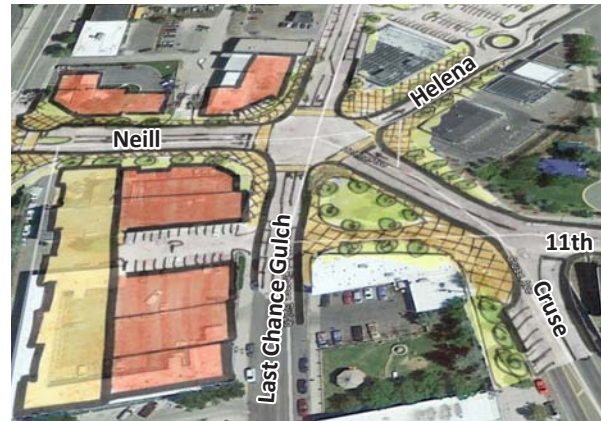
Reconfiguration of mini-malfunction junction is critical to restoring two-way traffic on Last Chance Gulch.
